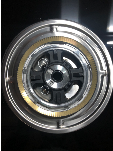
Step 1 - Remove the outer cap
